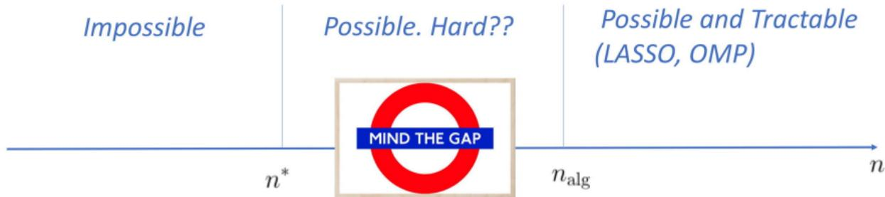
$$n^* = \frac{2k \log \frac{p}{k}}{\log(k/\sigma^2 + 1)}, n_{\text{alg}} = 2k \log \frac{p}{k}.$$
