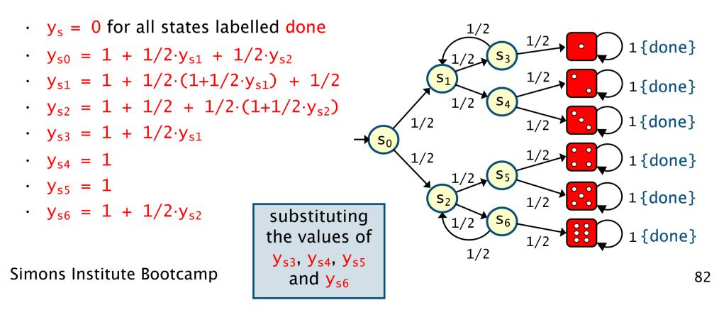
Expected number of coin flips if s is in T, then  $y_s = 0$ if s does not reach T with probability 1, then  $y_s = \infty$ otherwise  $y_s = r(s) + \Sigma_{s' \in S} P(s, s') \cdot R(s, s') + \Sigma_{s' \in S} P(s, s') \cdot y_{s'}$
