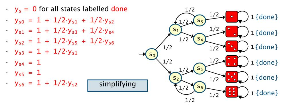
Expected number of coin flips if s is in T, then  $y_s = 0$ if s does not reach T with probability 1, then  $y_s = \infty$ otherwise  $y_s = r(s) + \Sigma_{s' \in S} P(s, s') \cdot R(s, s') + \Sigma_{s' \in S} P(s, s') \cdot y_{s'}$
