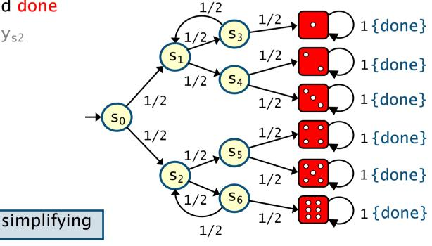
Expected number of coin flips if s is in T, then  $y_s = 0$ if s does not reach T with probability 1, then  $y_s = \infty$ otherwise  $y_s = r(s) + \Sigma_{s' \in S} P(s, s') \cdot R(s, s') + \Sigma_{s' \in S} P(s, s') \cdot y_{s'}$
