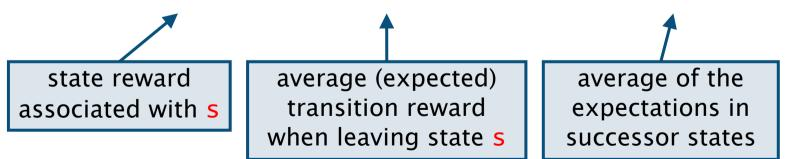
Expected number of coin flips if s is in T, then  $y_s = 0$ if s does not reach T with probability 1, then  $y_s = \infty$ otherwise  $y_s = r(s) + \Sigma_{s' \in S} P(s,s') \cdot R(s,s') + \Sigma_{s' \in S} P(s,s') \cdot y_{s'}$
